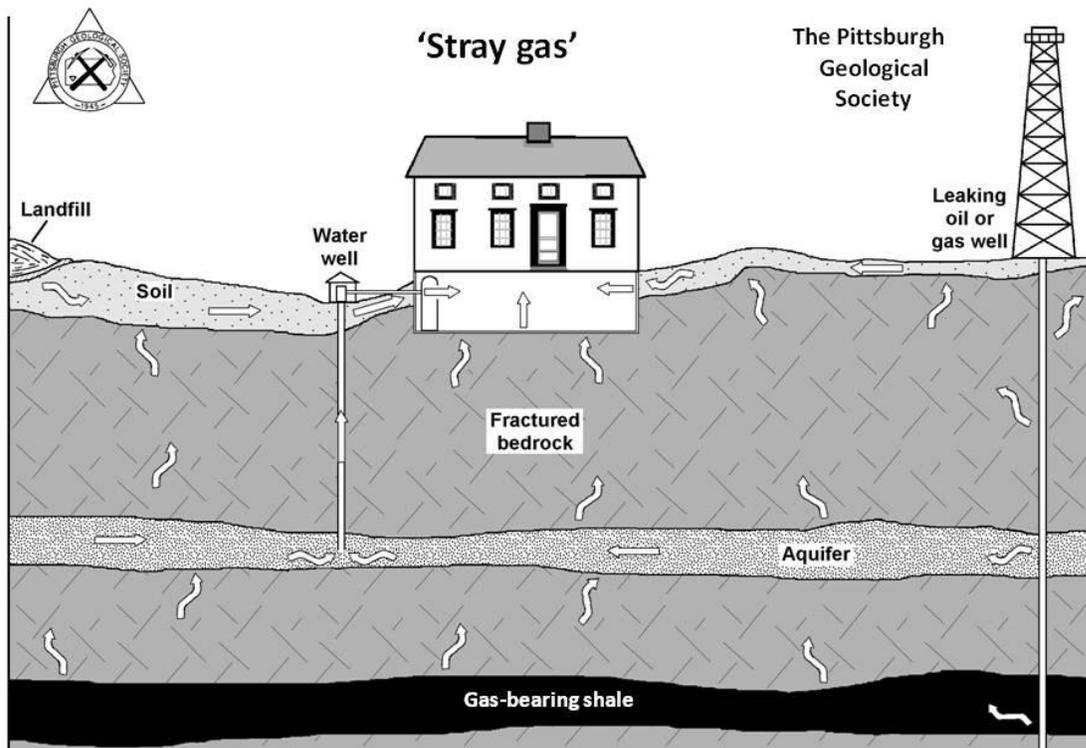
note: most stray gas in water wells migrates upward from depths of 10's to 100's of feet below the ground surface
